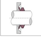
Improved lip designed to compensate shaft run-out
